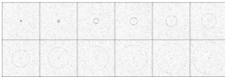
Figure 6. Spherical shock wave emitted by a sonoluminescing bubble into the surrounding liquid. The temporal separation of adjacent frames is ca. 30 ns; the frame size corresponds to an area of 1.6 \times 1.6 \text{ mm}^2 in the object plane.
