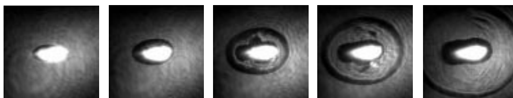
Figure 2. Bubble generation and shock wave emission upon laser-induced breakdown caused by a focused Nd:YAG laser pulse in water. The CCD photographs of the breakdown were taken with 100 fs pulses for back-illumination, obtained via a pulse picker from a Ti:sapphire laser. The frame size is 0.66 \times 0.66 \text{ mm}^2 . From left to right, the following time delays between the generating pulse and the illumination pulse apply (measured from peak to peak): 9.5 ns, 13 ns, 69 ns, 107 ns and 157 ns. The bright light emission is due to the laser-produced plasma. The forming bubble is visible as a dark border around the central spot. In the short time interval covered the bubble does not grow significantly.
